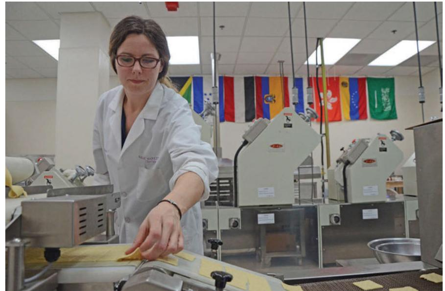
**SMALL-SCALE PRODUCTION:** Kathleen Gehring demonstrates the Wheat Marketing Center’s cracker line — where different levels of sugar, honey and other ingredients, as well as various blends of hard red winter and hard red spring, are used to test the flavor, texture, color and stackability of different crackers.
