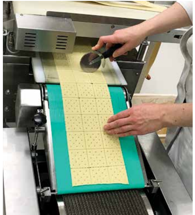
The cracker line at the Wheat Marketing Center in Portland is often used for research and product development. Here the crackers are heading into the three-part oven. Photo courtesy of the Wheat Marketing Center.
